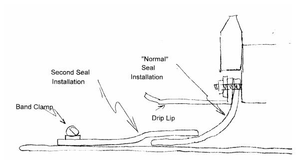
INSTALLATION "CROSS SECTION VIEW" OF SECOND INTRAMODULE SEAL ON G2 AND G3 MILNOR CBW.
